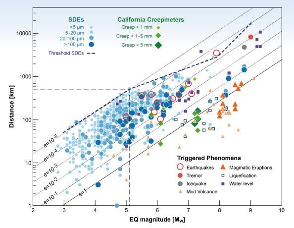
Triggered shallow slip observed on IPOC Creepmeters scale with seismic energy density and compare well with triggered slip observed on California Creepmeters. Both follow the same seismic energy density contours as other triggered phenomena.
